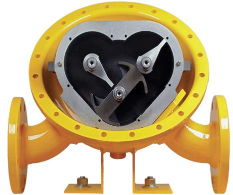
Because the force exerted by the fluid flowing through the meter is at right angles to the faces of the displacement rotors, and the rotor shafts are always in a horizontal plane, there is no axial thrust, thereby eliminating wear between the rotors and the bearing plates and ultimately providing a lifetime of measurement accuracy.
