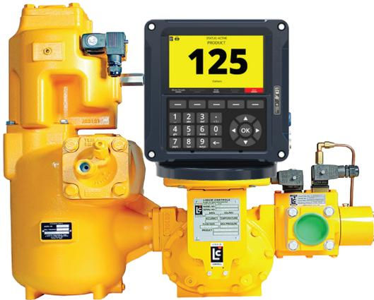
M-7® for refined fuels with LCR.iQ®, E-7 valve, optical air eliminator and high-capacity strainer.
