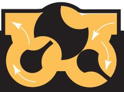
The original Liquid Controls tri-rotor meter design consists of a housing in which three rotors turn and measure fuel in synchronized relationship with no metal-to-metal contact.
